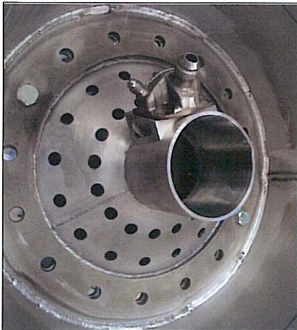
Nozzle and Diffuser. Inside view of the single-combustion liner test fixture shows dual fuel nozzle installation ready for steam-fuel mix testing.
