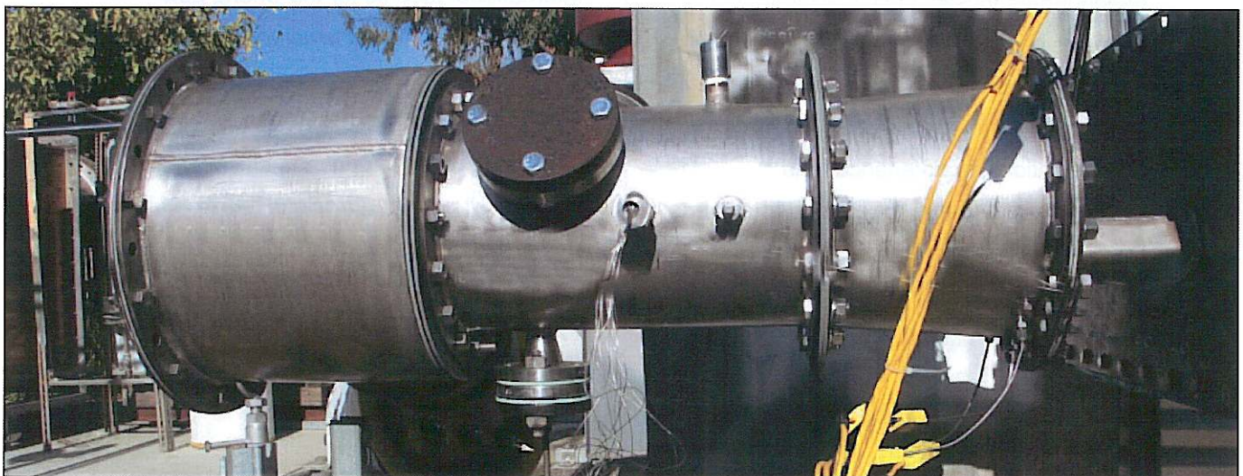
Test Stand. Combustion air (entering at the left) is preheated to the compressor discharge temperature of the 501KH to simulate gas turbine operating conditions. Rig testing follows similar testing performed by Cheng Power Systems to evaluate different gas turbine model applications.
